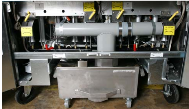
The levers on the right and left of the cabinet return oil through rear ports in the frypot. The center-mounted levers return oil through a top-mounted faucet. In all cases, a yellow lever returns oil to the frypot directly above it.
